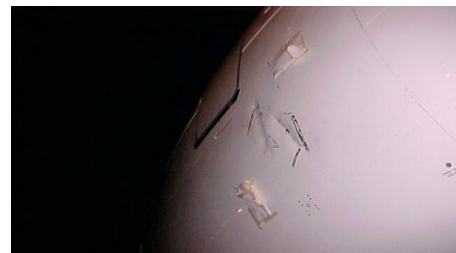
Figure 3 – Ground handling impact by passenger boarding bridge
