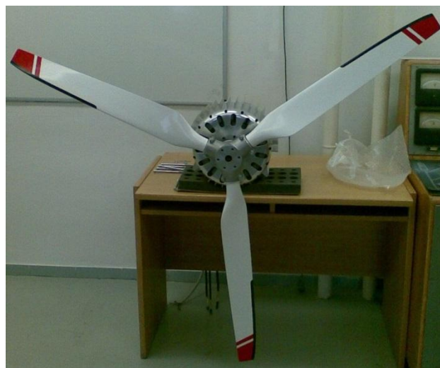
Figure 7 – Propeller with electric engine in laboratory
