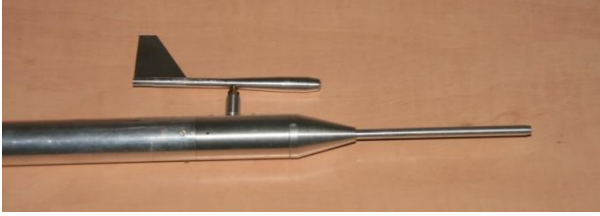
Figure 3 In-house developed angle of attack measurement probe
