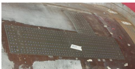
Figure 5 – Fuselage skin repair with large external doubler
