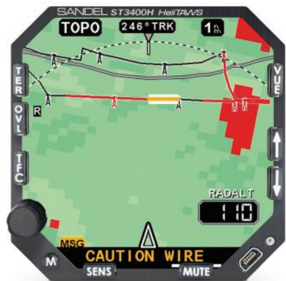
Figure 2 – Sandel HeliTAWS ST3400H, Wire warning [Source: HeliTAWS, Product description, ST3400H]
