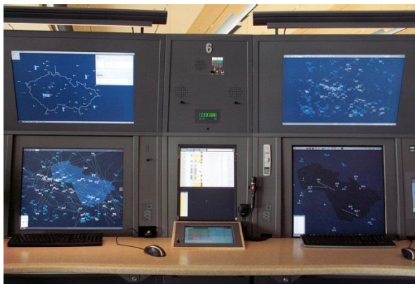
Figure 9 – Electronic flight strips at ACC Praha at IATCC Jenec - in the middle – primary electronic flight strips screen
