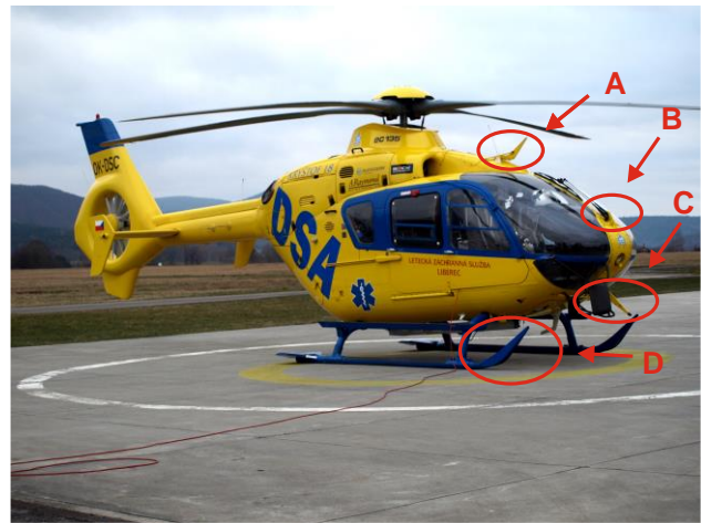
Figure 4 – Wire strike protection system with description of parts Conclusion
