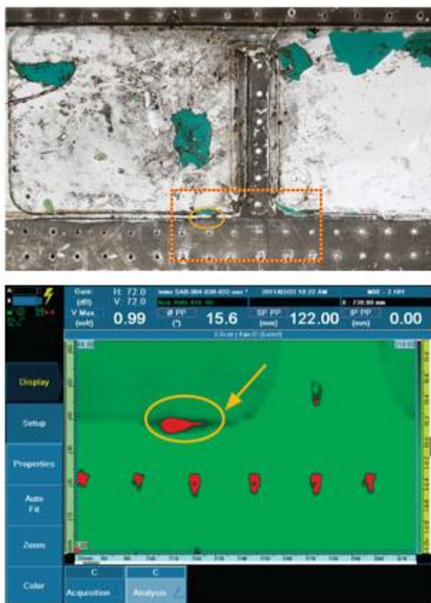
Figure 16 – Internal Subsurface Corrosion Area. Source : [9].
